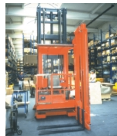
Side loading fork lift trucks run on Renold leaf chain are used to store and pick products in warehouses worldwide.
